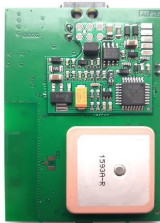
Picture 3. Navigation tracker Arnavi Integral 3 with the installed control module
